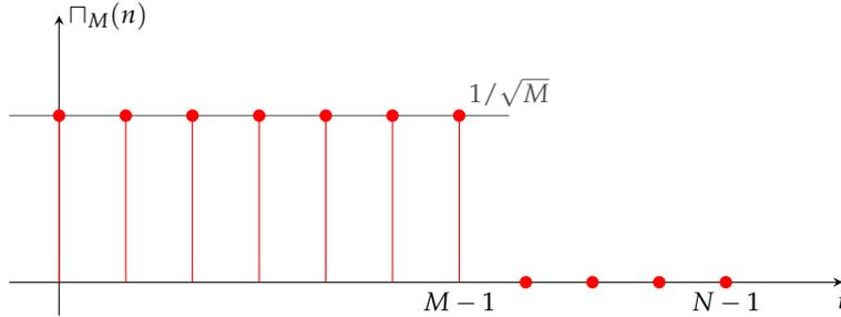
**Figure 1.** Unit energy square pulse of length  $T_0 = MT_s$  and duration  $T = NT_s$ . The signal is constant for indexes  $n < M$  and null for other  $n$ . The height of the pulse is set to  $1/\sqrt{M}$  to have unit total energy.
